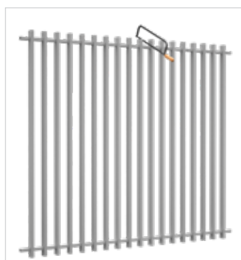
1 Cut panel to required width. NOTE: ensure minimum of 42mm of horizontal rail remains both sides past pickets for attaching of converters
